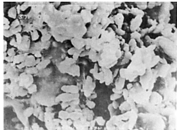
Figure 5 SEM of the ferric salt-loaded gelatin microcapsules by coacervation (magnification: 4.05K).
